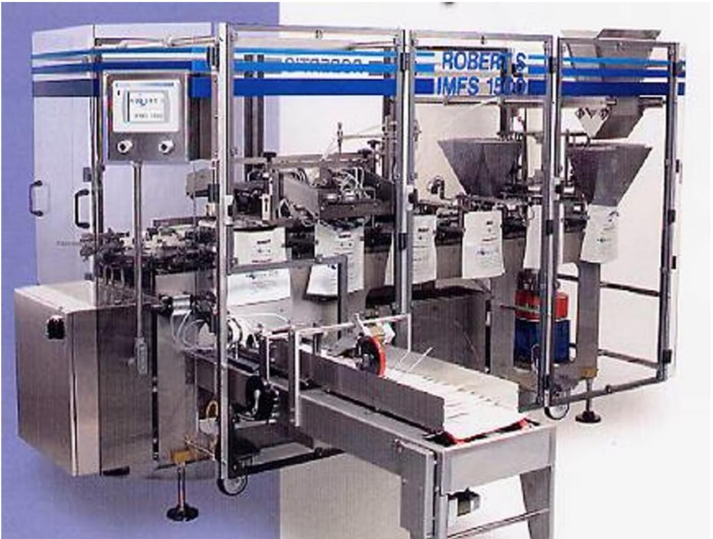
Stand-up pouch system automatically fills and seals premade standup/zipper style bags. Machine accommodates a minimum pouch size of 4" W x 6" H x 1" gusset through a maximum pouch size of 12" W x 15" H with a maximum gusset of 5". A complete size changeover can be performed in approximately 15 min. Benefits include a compact footprint, increased flexibility, and an economical price. Machine is built on the same construction criteria as Robert's C-Series continuous motion systems.
